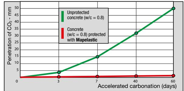
Fig. 2: Protection of Mapelastic against accelerated carbonation (30% of CO<sub>2</sub>) on porous concrete
